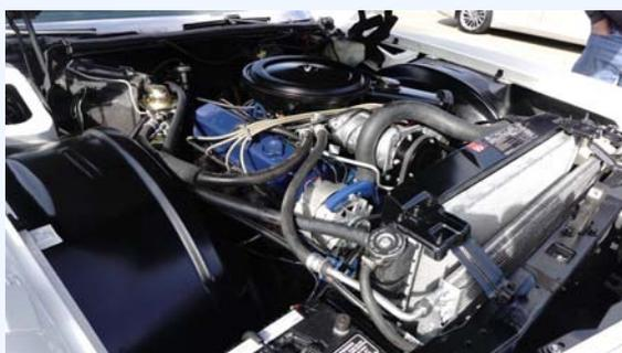
Jeff's highly detailed 500 cu in (8.2-liter) V8 engine, 190 horsepower and 360-pound feet of torque. 0-60 mph in 12.9 seconds, 0-100 mph in 42.9 seconds with a top speed of 115 mph.
