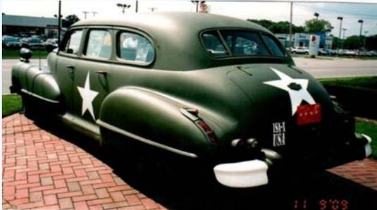
1942 Cadillac "Ike" staff car fully equipped Series 75, built by Fleetwood. In addition to the standard factory equipment that included a flathead V8, it has blackout shields for all of the lights, a siren and flag mounts. Everything on the outside is painted olive drab, including all of the chrome trim, hub caps, badging and hood ornament. It may be painted olive drab but the Cadillac crest and name is all over the car, every logo is intact.
